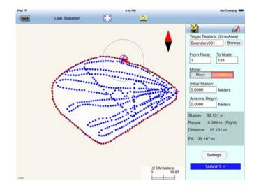
If you mark the checkbox for **Target Beep**, then when you are inside the target range, beeps will be sounded.
