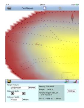
You may use the values displayed in the **Go** field to help ou reach the target. On the GPS marker, the solid grey arrow points in the direction you are moving, and the hollow blue arrow points in the direction of the Target. When you are moving in the right direction, these two arrows will coincide.
