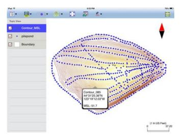
While the contour-regions map is displayed, the bubble that pops up when you tap in the contoured area will contain some information relevant to the contour-regions map. For example, when the contour-regions map generated by the Volume function is displayed, the bubble will provide the cut or fill information for the spot you tapped, and it will be referenced to the Base plane used in the Volume computation.
