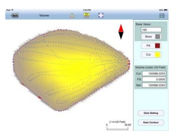
As you can see, with the **Base** set at the bottom of the pile, all of the volume is shown in the **Cut** field. This means that if you were to bring the pile to the ground level, this much of it needs to be removed (or cut).
