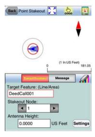
You can select which Node you would like to stakeout. Type in the desired Node #, or tap the little right arrow button to change the Node # to another
