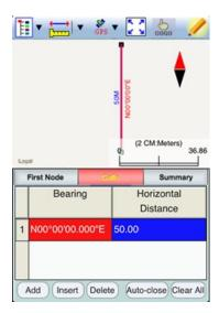
If you need to change the data entered for any record, simply double-tap on the record to call up the data entry screen then enter the correct data.
