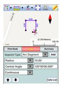
Tap the Calls List button to see the Deed Calls records. You may tap the Insert button to insert a record before the highlighted record, tap the Delete button to delete the highlighted record, or tap the Clear All button to clear all existing deed calls from the list and start a new deed call drawing.
