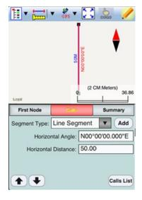
First, specify the type of segment you will be adding. Choose between **Line Segment** for straight lines or **Arc Segment** to define an arc.
