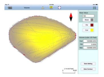
As you can see, with the **Base** set at the bottom of the pile, all of the volume is shown in the **Cut** field. This means that if you were to bring the pile to the ground level, this much of it needs to be removed (or cut).
