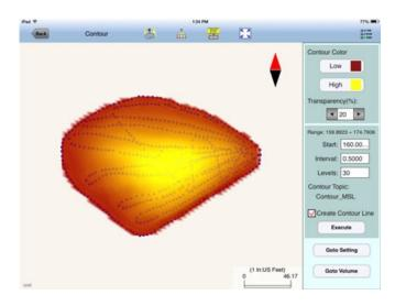
If you don't want the contour lines displayed, then unmark the check box for "Create Contour Line" and tap the "Execute" button.
