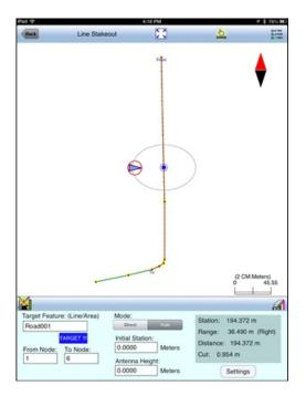
If you mark the checkbox for **Target Beep**, then when you are inside the target Tolerance range, beeps will be sounded.
