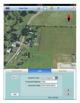
First, specify the type of segment you will be adding. Choose between **Line Segment** for straight lines or **Arc Segment** to define an arc.
