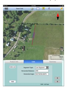
First, specify the type of segment you will be adding. Choose between **Line Segment** for straight lines or **Arc Segment** to define an arc.
