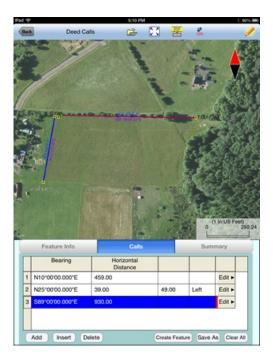
Whenever the Deed Calls records are displayed, you may tap the **Insert** button to insert a record before the highlighted record, tap the **Delete** button to delete the highlighted record, or tap the **Clear All** button to clear all existing deed calls from the list and start a new deed call drawing.
