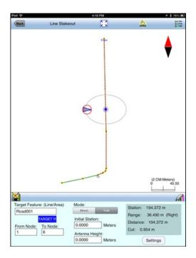
If you mark the checkbox for **Target Beep**, then when you are inside the target Tolerance range, beeps will be sounded.
