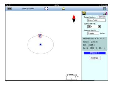
If you mark the checkbox for **Target Beep**, then when you are inside the target Tolerance range, beeps will be sounded.
