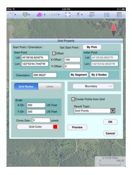
The **Start Point** section lets you specify the reference location for the grid. You may enter the coordinates for that point or tap the **By Pick** button to select the location from Map View. If the reference point is a known point but you want to shift the grid a distance from it then tap the **Offset** checkbox to display the relevant data entry fields. The software will compute the new grid reference point based on the offset entered.
