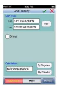
Tap the **Pick** button then tap on the displayed map to select a starting point for the grid.
