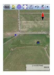
If your device has GPS capability, you could add a point right at the current GPS position. To do so, first tap the **Down Arrowhead** at the upper-right corner of the screen and select **GPS ON** to turn on GPS then tap the **Pick**
