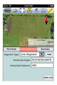
First, specify the type of segment you will be adding. Choose between **Line Segment** for straight lines or **Arc Segment** to define an arc.
