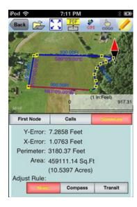
Options are provided to perform an adjustment using the compass method or the transit method.
